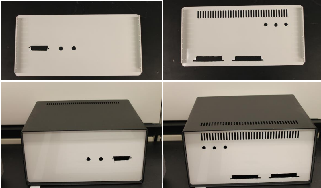
Figure 5 - Front panel (top left) and back panel (top right) with holes cut out. Front panel (bottom left) and back panel (bottom right) secured within the box.
