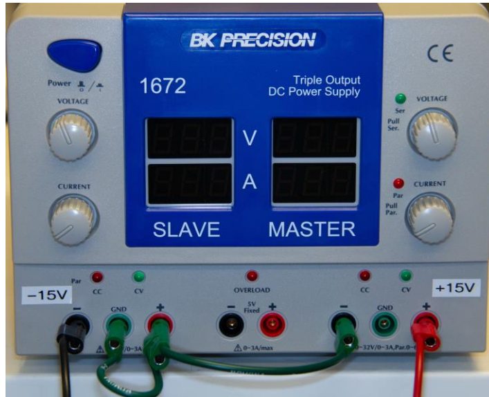
Figure 1 - Power supply configuration.
